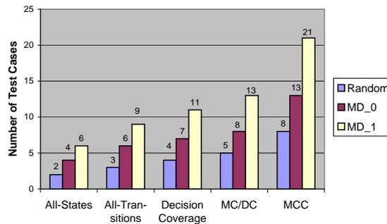
Figure 3.32: Test suite sizes for the elevator control example.
