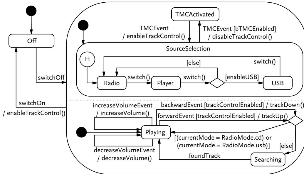
Figure 5.4: A state machine describing an extract of the general car audio system behavior.
