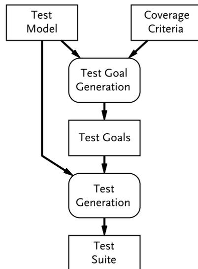
Figure 1.1: Model-based test generation.
