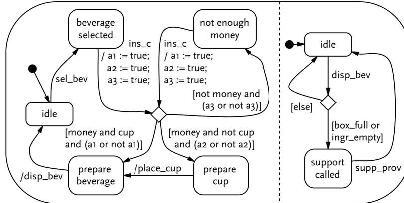
Figure 4.24: Transformed test model to simulate All-Uses with All-Defs.
