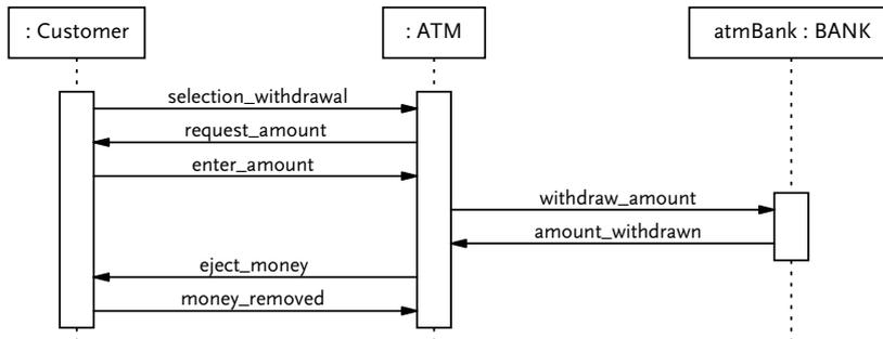
Figure 5.14: Sequence 2: Interaction diagram for withdrawing money.
