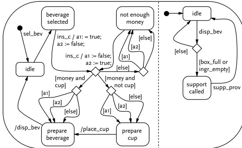
Figure 4.22: Transformed model to simulate All-Uses with All-Transitions.
