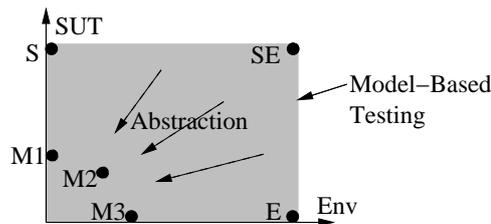
Figure 2.14: Test models describe the SUT or its environment according to Utting, Pretschner, Legnard [UPL06] (used with permission).
