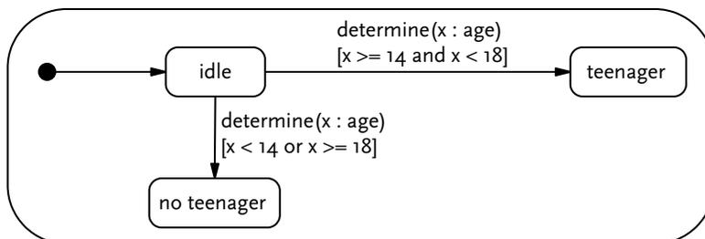
Figure 3.11: State machine describing the reaction to the input values of the teenager partitioning.
