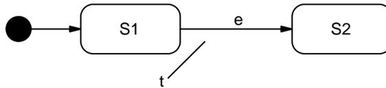
Figure 2.16: State machine example to clarify definitions of coverage.
