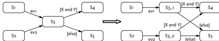
Figure 4.36: Example for a model transformation to support the level-3-combination of control-flow-based and transition-based coverage criteria.
