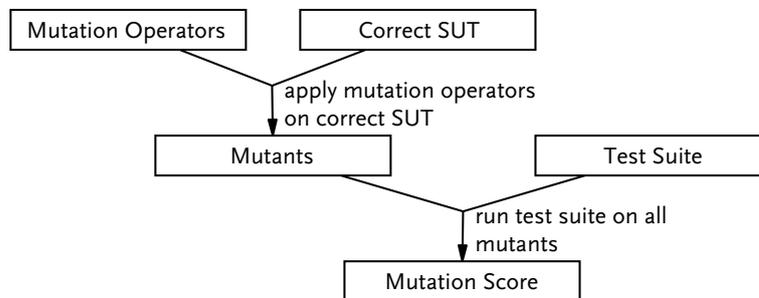
Figure 2.7: The basic process of mutation analysis.
