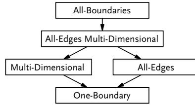
Figure 2.6: Subsumption hierarchy for boundary-based coverage criteria.
