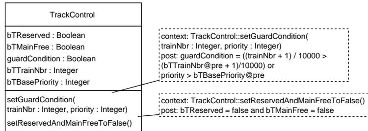
Figure 3.20: Class diagram of the track control.
