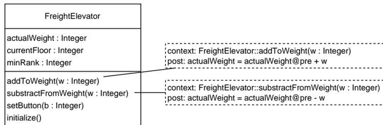
Figure 3.15: Class diagram of the freight elevator control.
