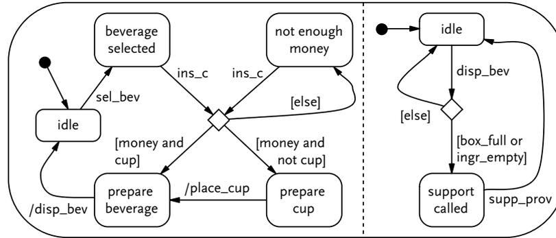
Figure 4.15: UML state machine describing the behavior of a coffee dispenser.
