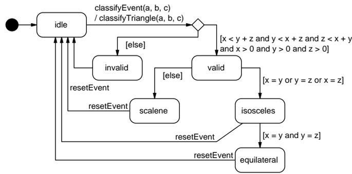
Figure 3.17: State machine for the triangle classification.
