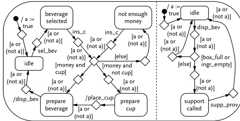
Figure 4.30: Transformed test model to simulate All-Transitions with Condition Coverage.
