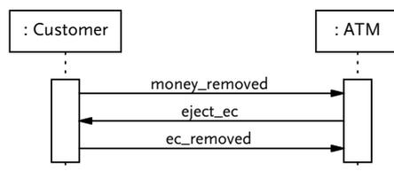
Figure 5.15: Sequence 3: Interaction diagram for removing money and EC card.
