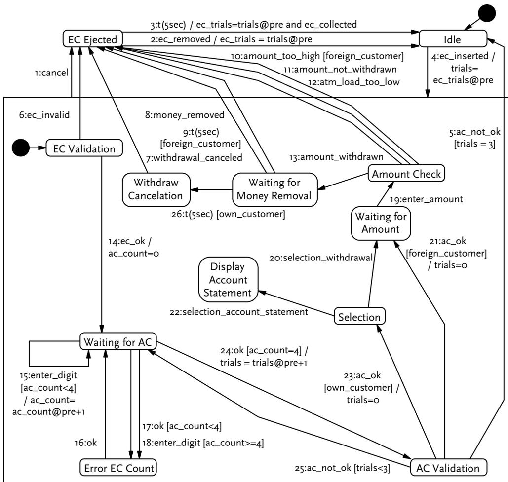
Figure 5.12: State Machine of ATM
