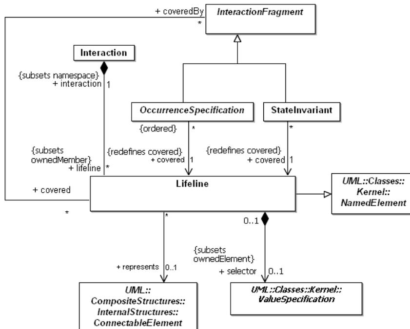
Figure 2.10: Meta model for interactions and life lines (UML 2.1).
