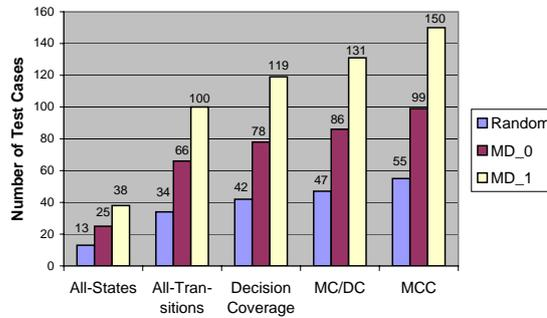
Figure 3.38: Test suite sizes for the train control example.
