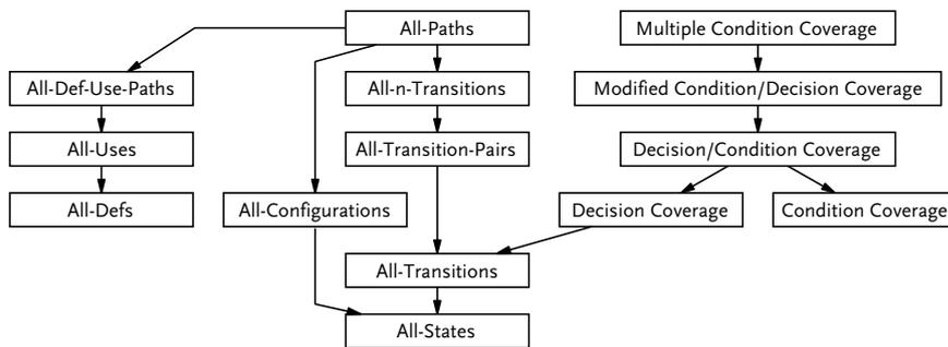
Figure 2.5: Subsumption hierarchy for structural coverage criteria that are focused on transitions, control flow, and data flow.
