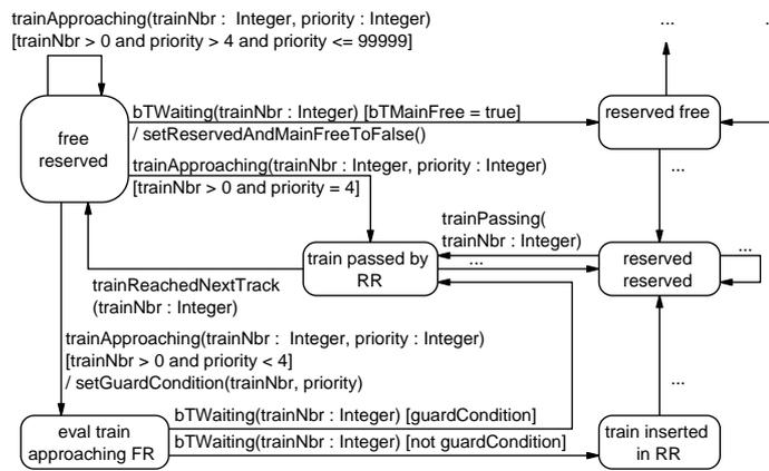
Figure 3.19: State machine of the track control.
