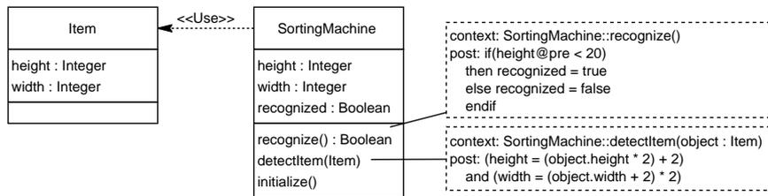
Figure 3.13: Class diagram of a sorting machine.
