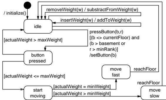
Figure 3.14: State machine of the freight elevator control.
