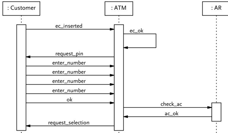
Figure 5.13: Sequence 1: Interaction diagram for inserting the EC card.
