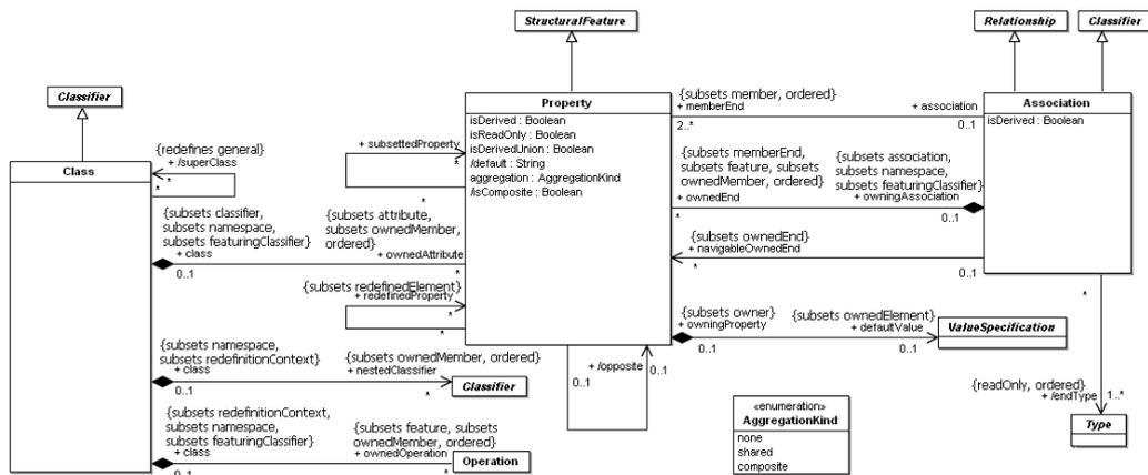
Figure 2.9: Meta model for classes (UML 2.1 specification).
