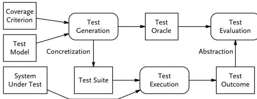
Figure 2.12: Concretization and abstraction in model-based testing.
