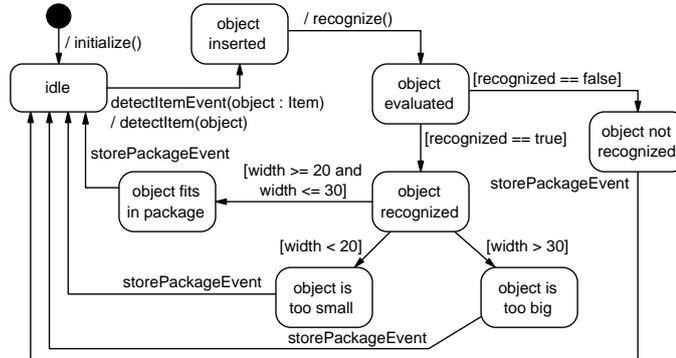
Figure 3.27: State machine of a sorting machine.
