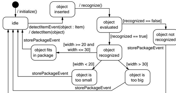
Figure 3.12: State machine of a sorting machine.
