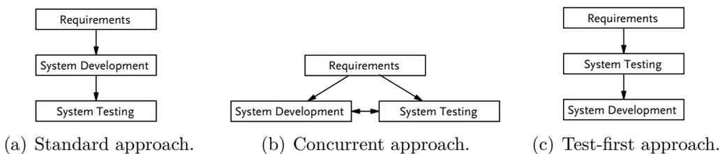
Figure 2.4: Different approaches to integrate testing into system engineering.
