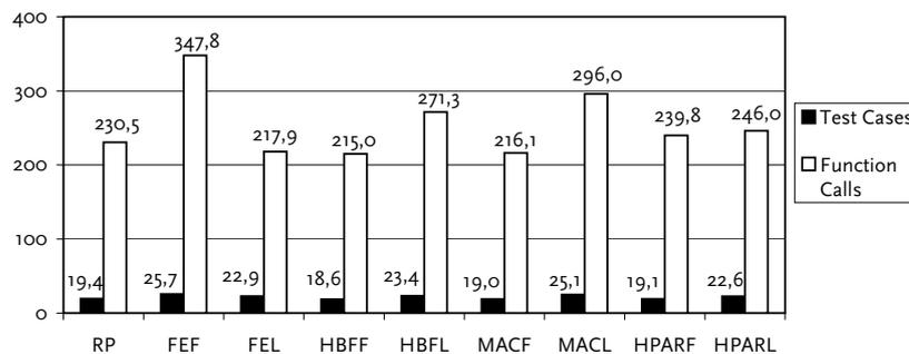
Figure 6.7: Average test effort for SPS and offline testing for masking MC/DC.
