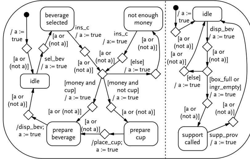
Figure 4.32: Transformed test model for the simulated satisfaction of All-Transitions with All-Defs.
