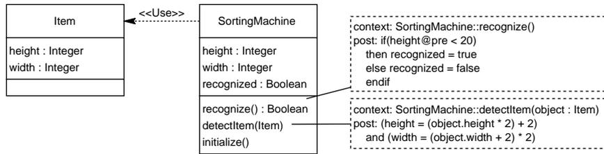
Figure 3.28: Class diagram of a sorting machine.
