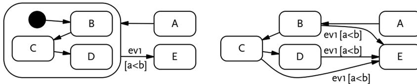
Figure 4.2: Hierarchical and flat state machine.
